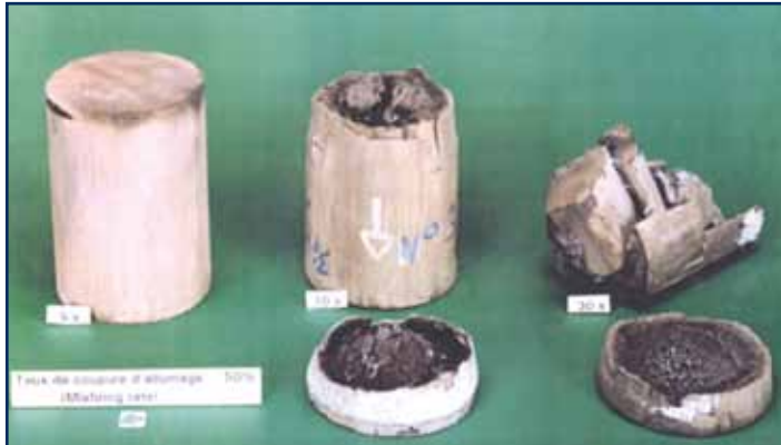
Three-way catalyst with ceramic substrate after 5, 10 or 30 seconds of work on engine bench with 50% ignition failures.
